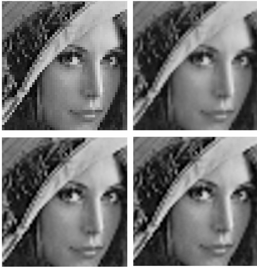
Fig. 5. Comparison with different interpolation techniques. Top left: nearest neighbor interpolation. Top right: bilinear interpolation. Bottom left: cubic spline interpolation. Bottom right: interpolatory subdivision scheme.
